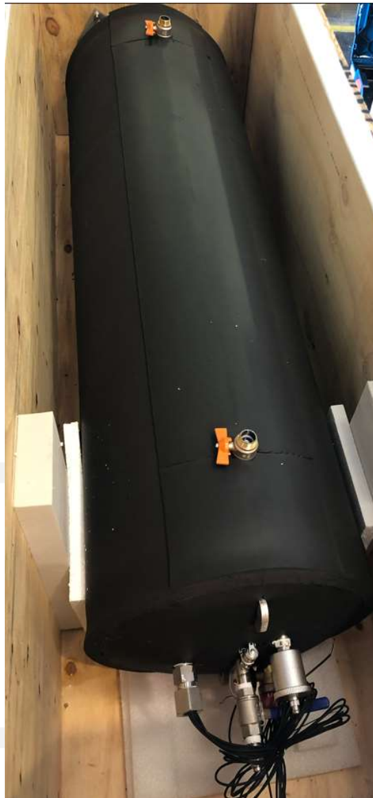
Figure 5. TCM reactor ready to be delivered with insulation jacket installed.
