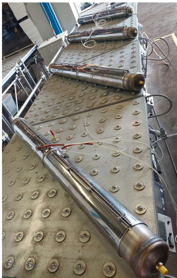
Figure 2. Reactor tubes finished and ready to meet TCM reactor.
