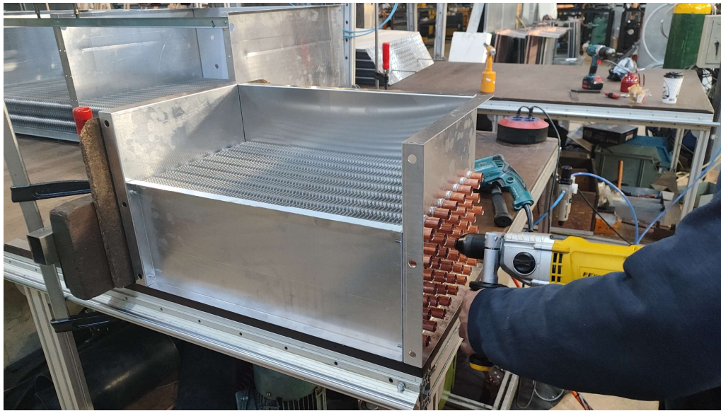
Figure 22. Manufacturing of the fan coil for the Ministor system.
