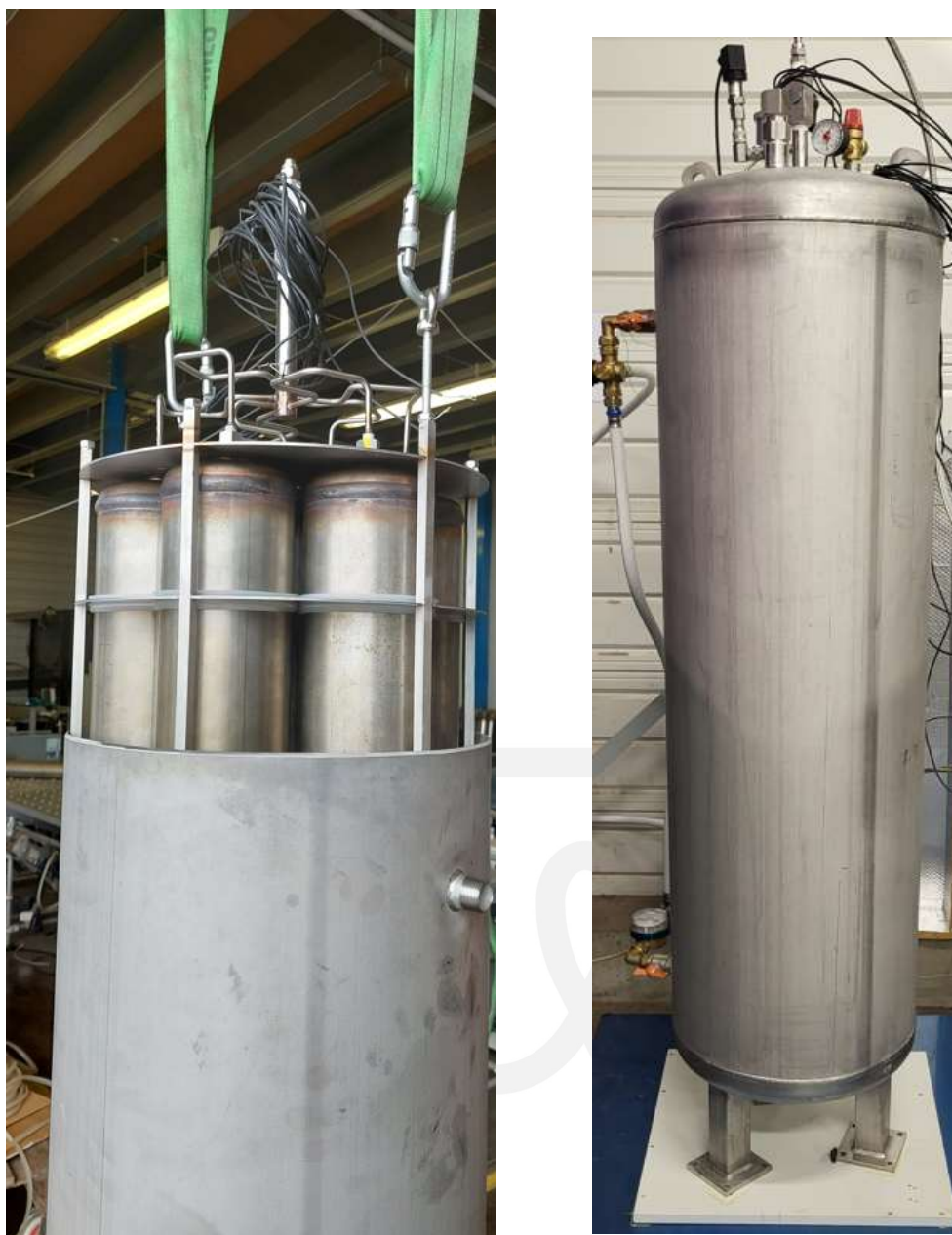
Figure 3. TCM assembly (left) and the completed TCM (right).
