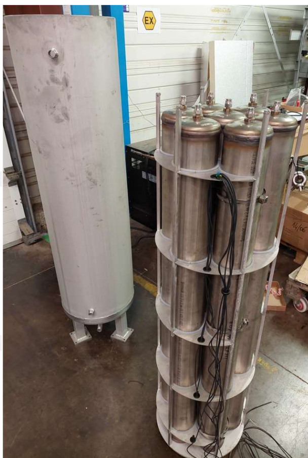
Figure 2. Reactor tubes finished and ready to meet TCM reactor.
