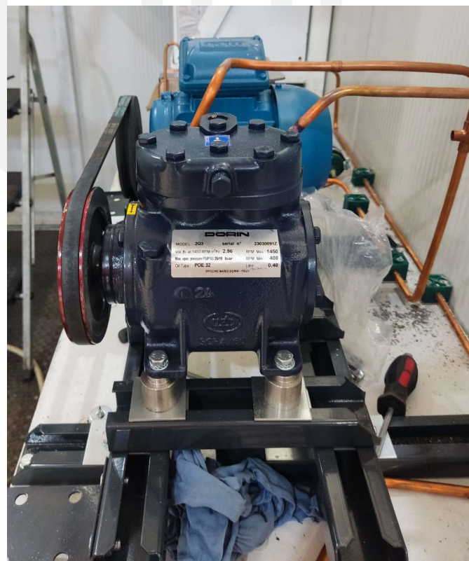
Figure 21. Dorin compressor for R134a used for the heat pump.
