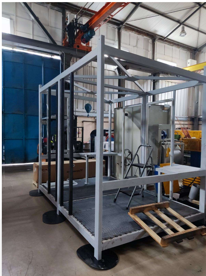
Figure 6. The metal frame of the MiniStor container at the premises of Psycrotherm.
