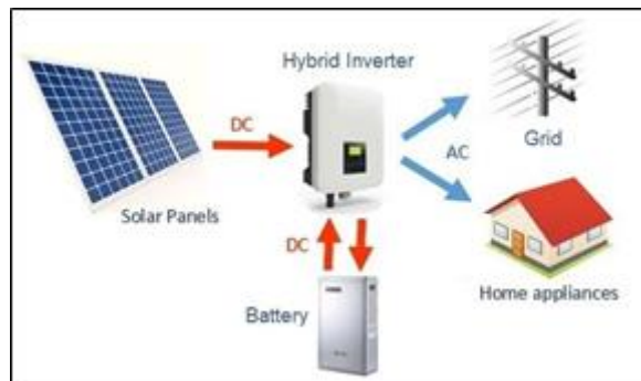
Figure 34: Connection of PVT Solar Array, Inverter and Battery to the house and the mains of Cork demo site
