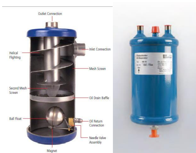
Figure 17: Hermetic oil separator manufactured by ESK-Shulze ( www.esk-schultze.de )
