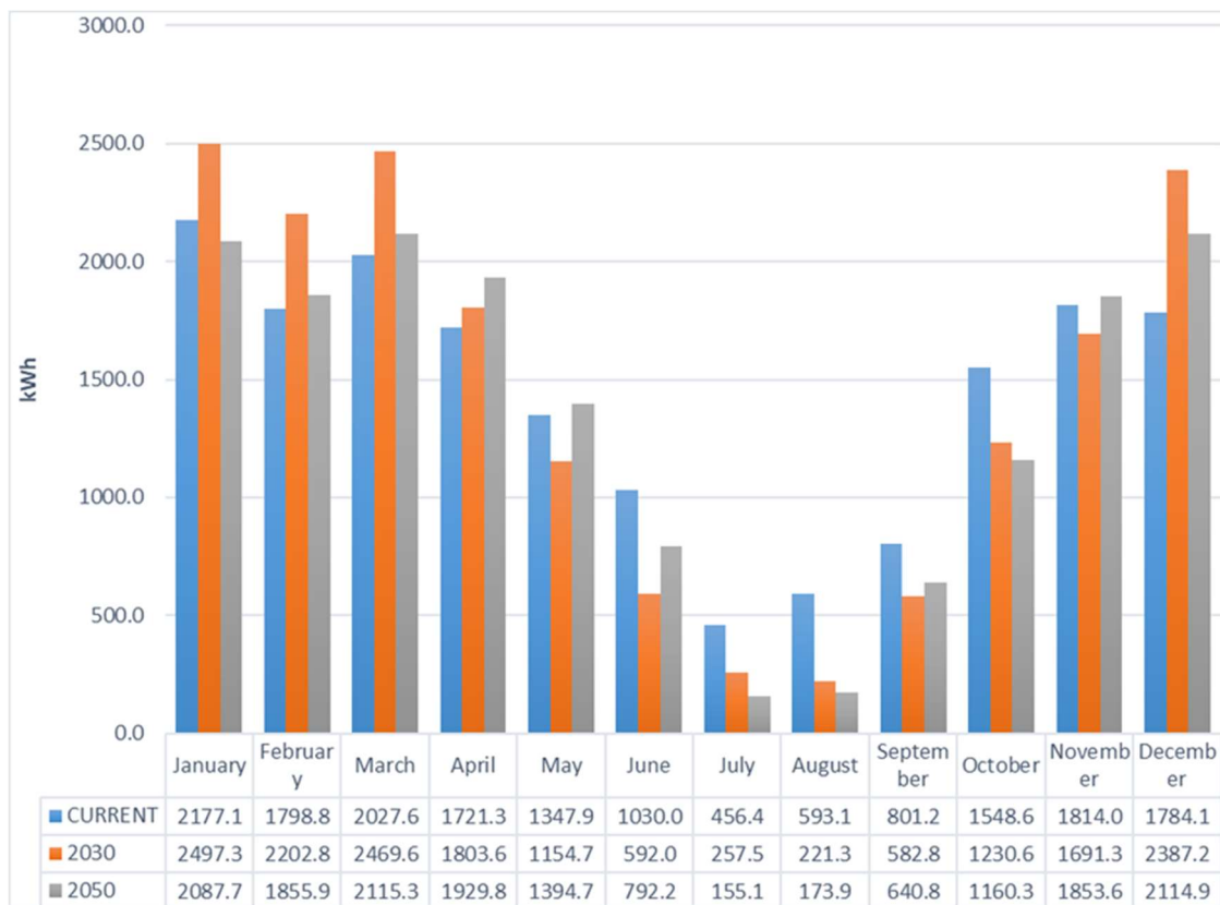
Figure 7 Monthly thermal loads in current year, 2030 and 2050 for Cork (Ireland) demo site
